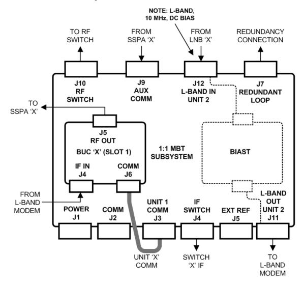
Figure 1-2. MBT-4000B Typical Application Schematic
