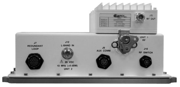
Figure 3-4. MBT-4000B External Connectors – RF Signal Side
