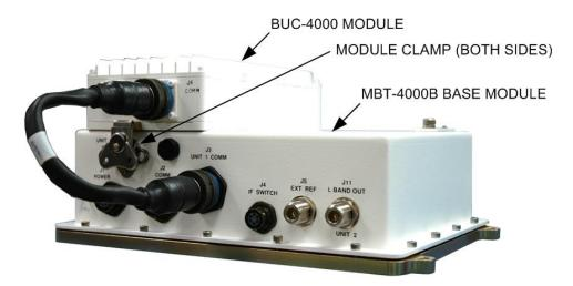
Figure 2-1. MBT-4000B Multi-Band Transceiver System Components
