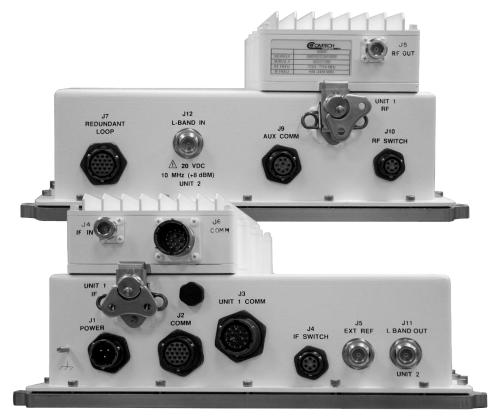
(TOP) IF Side (BOTTOM) RF Side – Cable Loop Removed for Clarity
