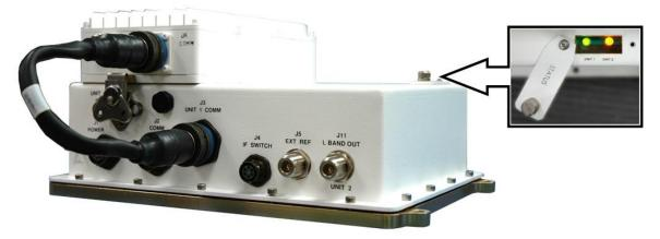
Figure 4-1. MBT-4000B Multi-Band Transceiver LED Indicators
